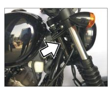
The frame serial number is stamped on the right side of the steering head tube.
