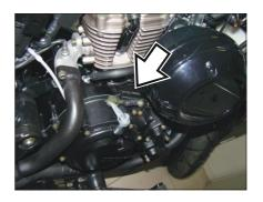
The engine serial number is stamped on the right upside of the crankcase assembly.
