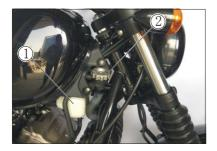
The right side of the front end of the vehicle fuel tank is provided with a white makeup water tank ① and a radiator cover ②.
