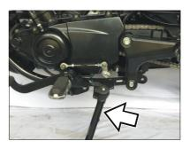
The motorcycle is equipped with the side stand ignition interlock system.
