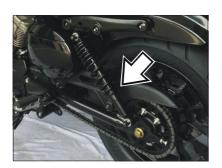
To adjust the spring pre-load, turn the adjuster clockwise or count- er-clockwise to the desired position with the pin spanner.
