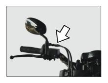
Always check the status of the cable's rubber cap assembly and must be assembled in the correct position.
