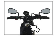
To open the fuel tank cap, insert the ignition key into the cap lock and turn it clockwise. With the key inserted, pull back the fuel tank cap.
