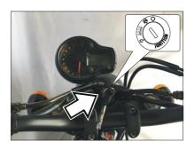
The ignition switch is located on the dashboard below.
