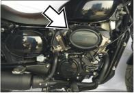
If the air cleaner element has become clogged with dust, intake resistance will be increased, as a result decrease in output power and increase in fuel consumption.
