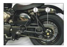
Place a jack or block under the swing arm to lift the rear wheel slightly off the ground.
